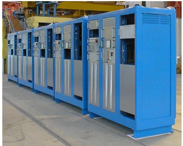
Fig. 173. Production series of 66 kV RCPSs near completion.
